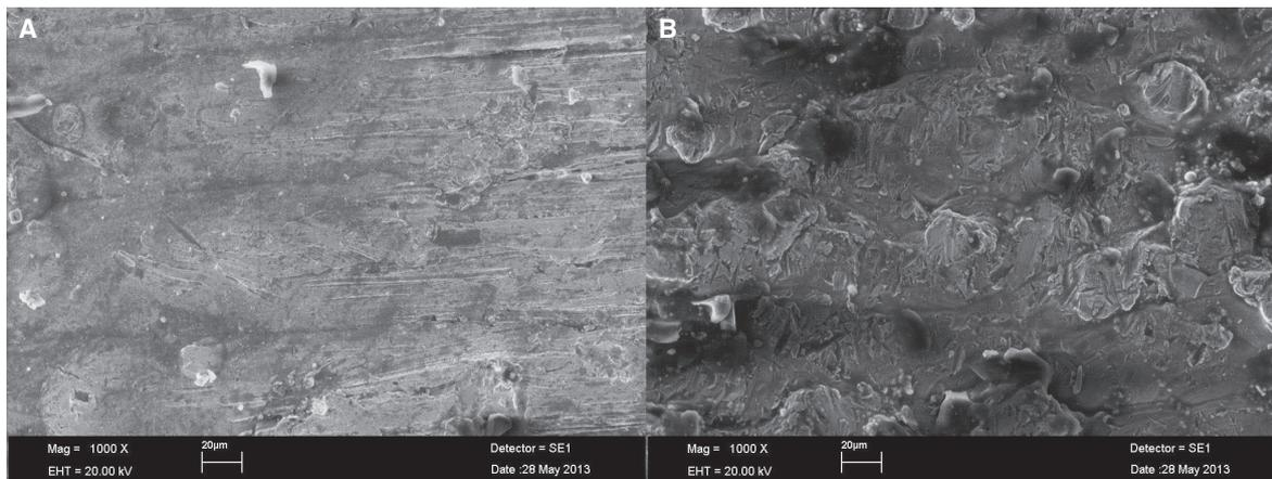
**Fig. 5.** ×1000 images of (A) Galvano coping surface and (B) Laser sintered Co-Cr coping surface.
