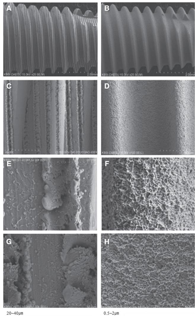
**Fig. 3.** Experimental and control group implant images obtained by field emission SEM: (A) Experimental group (×25); (B) control group (×25); (C) experimental group (×150); (D) control group (×150); (E) experimental group (×1,000); (F) control group (×1,000); (G) experimental group (×1,000); (H) control group (×1,000).
