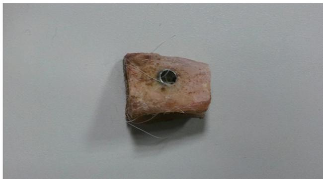
**Fig. 2.** Tibia sample including the inserted implant.
