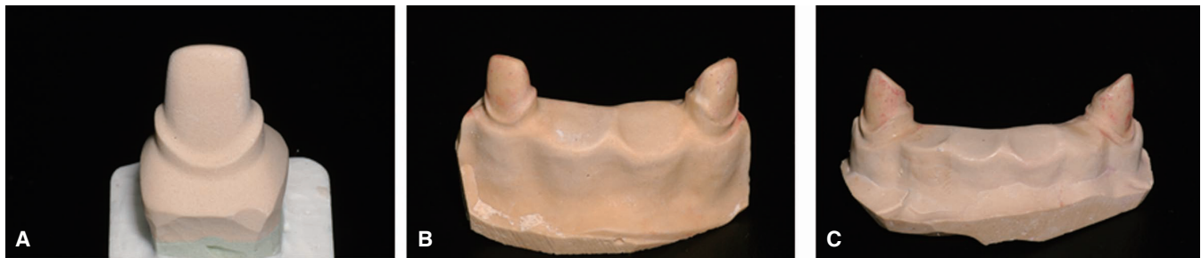
Fig. 2. Duplicated master models with dental stone. A: single, B: 4-unit, C: 6-unit.
