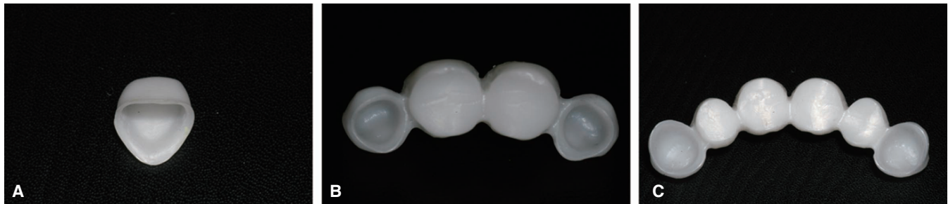
Fig. 3. Zirconia cores fabricated using CAD/CAM (Orapix, Seoul, Korea). A: single, B: 4-unit, C: 6-unit.
