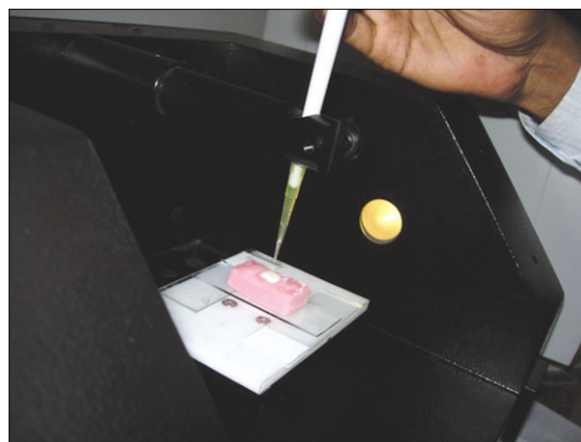
Fig. 8. "Deionized" water placed using pipette.
