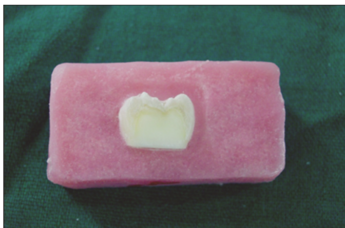
Fig. 1. Dentin exposed coronal portion of tooth mounted in autopolymerizing resin block.
