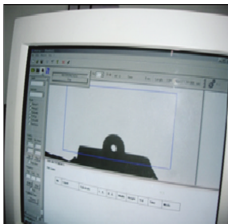
Fig. 9. Contact angle values as seen in the computer.
