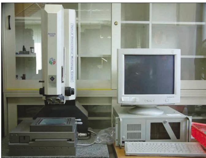
**Fig. 4.** The light microscope with image processing (Accura 2000).
