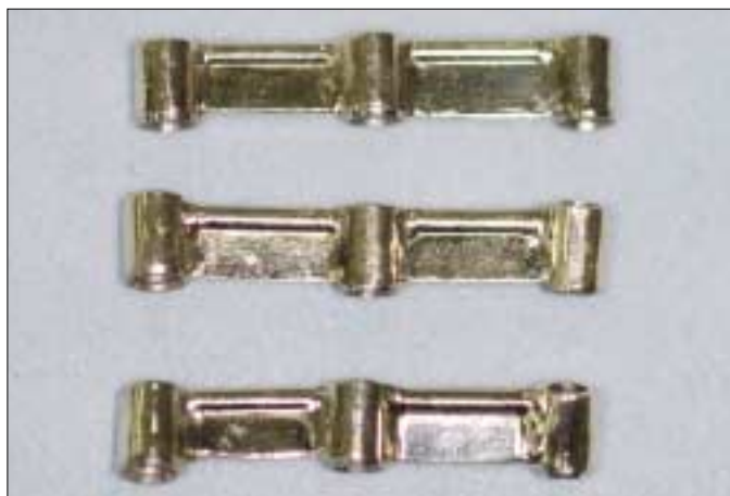
Fig. 1. Reference frameworks were waxed and cast on preliminary casts. Top: 0 degree, middle: 30 degrees, bottom: 40 degrees.
