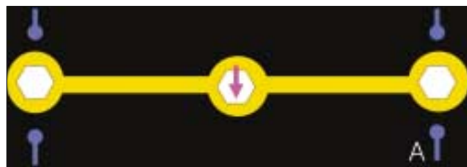
Fig. 5. Schematic drawings of the position and direction of measurement for statistical analysis. The arrows represent the screw tightening position and the round arrows represent measurement positions. A: Screw tightening of center analog and measurement of outer analogs, B: Screw tightening of left analog and measurement of right analog; screw tightening of right analog and measurement of left analog.
