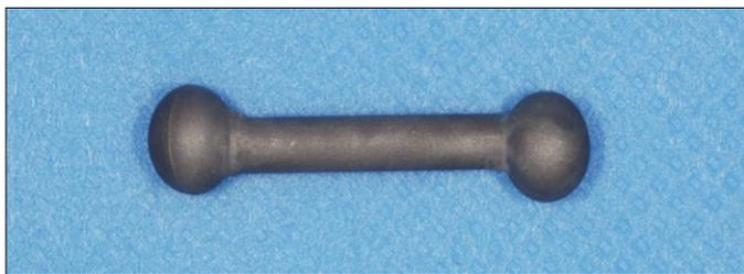
Fig. 1. The specimen made with Ni-Cr alloy.
