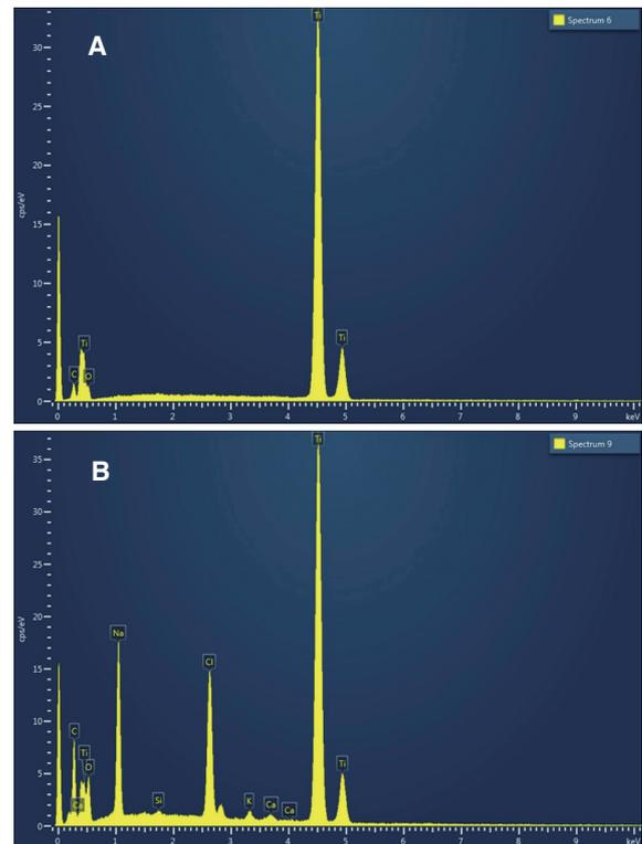
**Fig. 2.** (A) LE implant EDS spectrum. Ti, O, and C were the only three elements found in the LE implant surfaces. (B) modSLA implant EDS spectrum. Na, Ca, Cl, and K were also observed in modSLA, in addition to Ti, O, and C.
