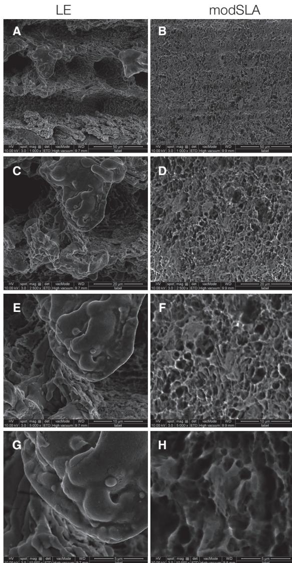
**Fig. 1.** Scanning electron microscopy image of LE and mod SLA implant surfaces. (A)  $\times 1,000$ , (B)  $\times 1,000$ , (C)  $\times 2,500$ , (D)  $\times 2,500$ , (E)  $\times 5,000$ , (F)  $\times 5,000$ , (G)  $\times 10,000$ , (H)  $\times 10,000$ .
