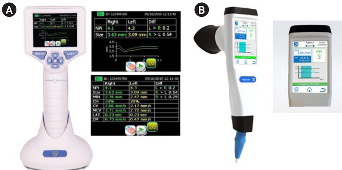
**Fig. 2.** Quantitative pupillometers devices and parameters. (A) NeuroOptics NPITM-200 and result screens. (B) NeuroLight-Algiscan and result screen. Reproduced from NeuroOptics (<https://neurooptics.com/npi-200-pupillometer>) and IDMED (<https://www.idmed.fr/en/analgesia>) with permission.
