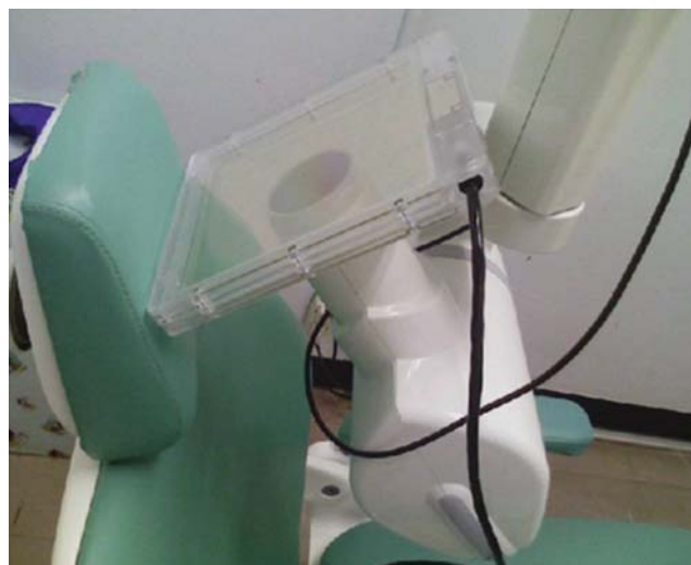
Fig. 1. The ionization chamber of DAP meter is positioned at the end of the exit cone of the intraoral X-ray machine for PED and DAP measurement.
