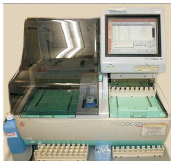
Fig. 1. A complete picture of the OC-sensor DIANA. The equipment can measure up to 150 samples in a single session.
