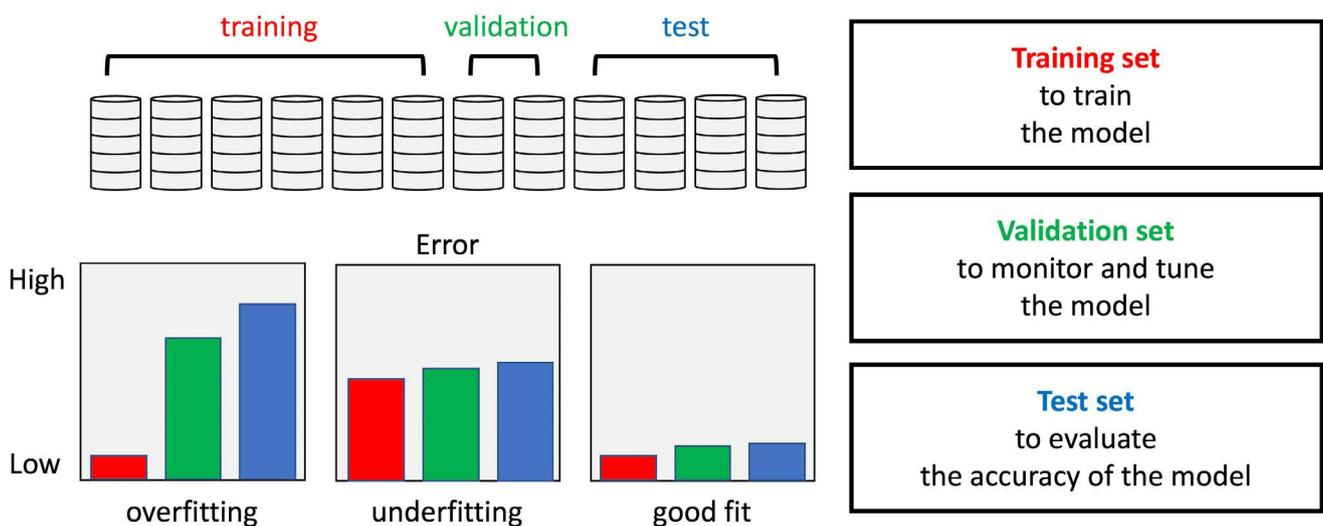
**Fig. 3.** Splitting data into training, valid, and test sets is generally recommended so as to avoid overfitting and evaluate the performance objectively. The optimally fitted network shows similarly good performances for all three data sets.
