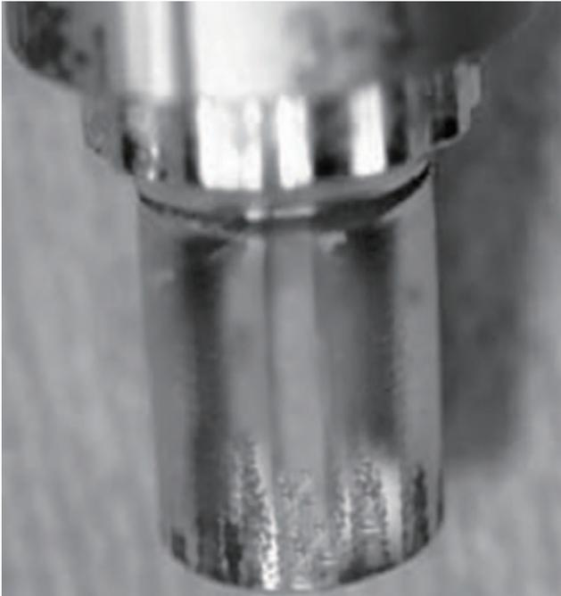
**Fig. 2.** Photo of the neck component demonstrates the corrosion.
