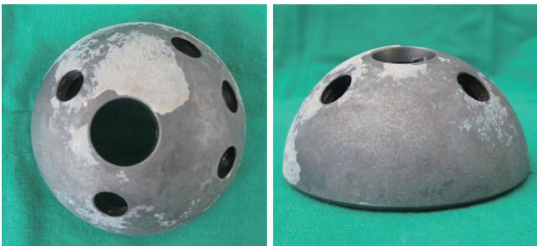
**Fig. 4.** The acetabular cup, which was retrieved at 4 years after index operation, showed extensive loss of hydroxyapatite coating.
