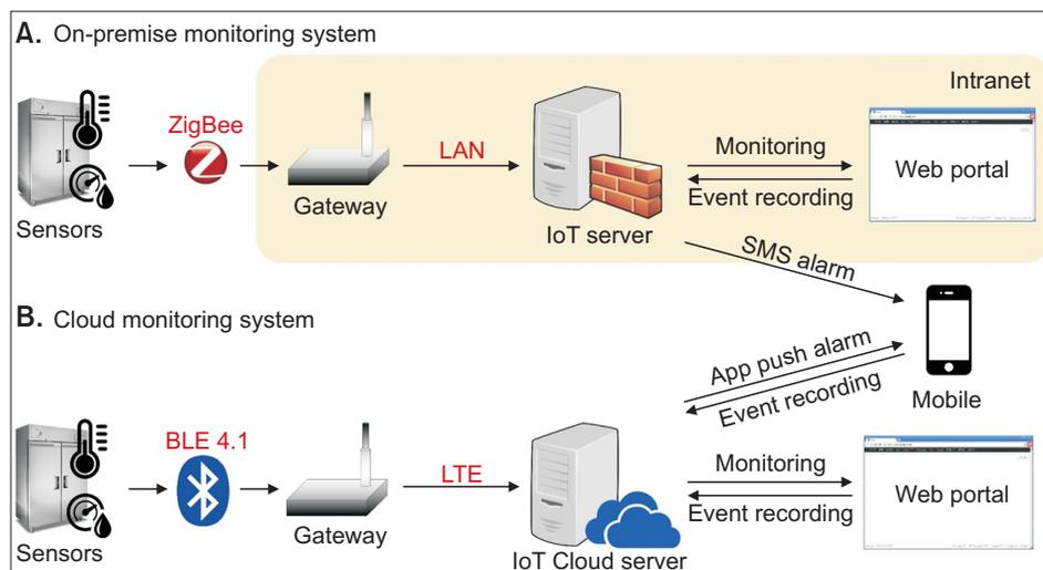
Figure 1. Architecture of both environmental monitoring system types. (A) On-premise monitoring system. (B) Cloud monitoring system.
