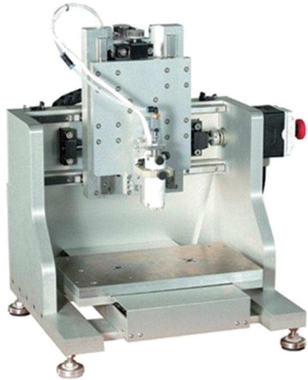
**Fig. 1.** 3D bio-printer available in Korea (given by KIMM). Hydrogel and cells can be injected by bio-printer with pre-determined CAD program and tissue with cells and biodegradable polymer can be made.
