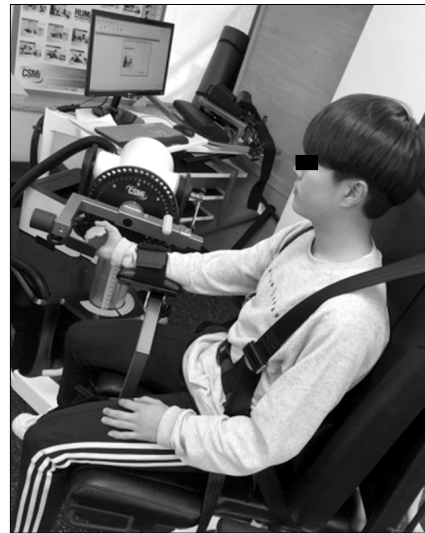
Fig. 2. Measure of wrist flexion and extension isokinetic strength.
