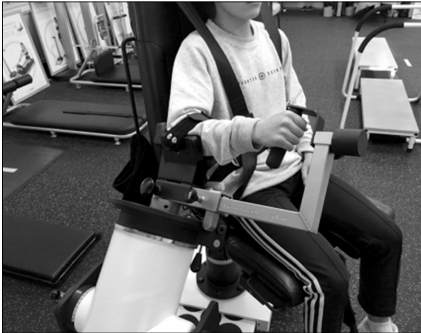
Fig. 1. Measure of shoulder internal rotation and external rotation isokinetic strength.
