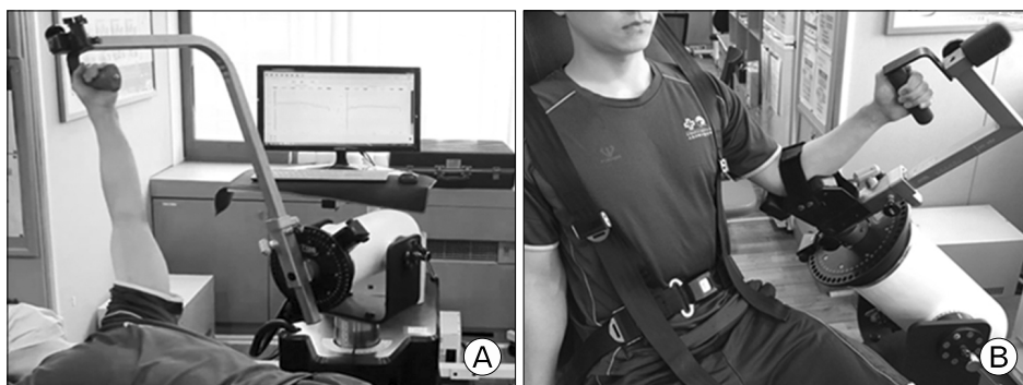
Fig. 3. Evaluation of shoulder isokinetic strength. (A) Forward flexion/extension. (B) External/internal rotation.
