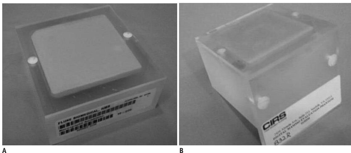
**Fig. 1. Two mammography accreditation phantoms.** Left is ACR Phantom (Nuclear Associates model 18-220) and right is Digital Phantom (CIRS Model 015DM). Digital Phantom has extended top edge allows ease of positioning on recumbent biopsy units. **A.** ACR Phantom. **B.** Digital Phantom. ACR = American College of Radiology
