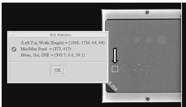
**Fig. 2. Calculation of signal to noise ratio (SNR).** Radiologist drew square-shaped region of interest (arrow) in background of phantom and then recorded mean value of SNR and standard deviation. SNR values were calculated based on following equation:
