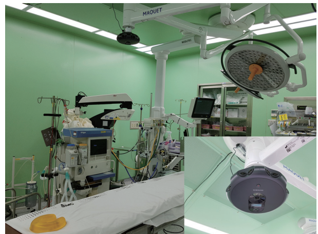
Fig. 7. VR camera for facial plastic and reconstruction surgery (360 round, Samsung electronic company, Seoul, Korea) which is installed in Samsung Changwon Hospital operating room. With 17 lenses, it is possible to record high-resolution images and implement VR environment. VR: virtual reality.
