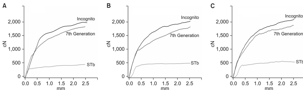
**Figure 4.** Comparison of frictional forces among the 3 lingual bracket types under the same displacement condition. **A**, Control, no displacement. **B**, 1-mm palatal displacement of the maxillary right lateral incisor. **C**, 1-mm gingival displacement of the maxillary right canine.
