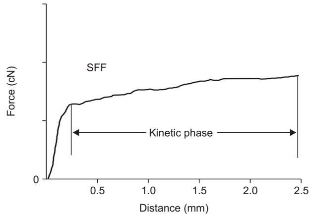
**Figure 3.** Definitions of static (SFF) and kinetic frictional forces (KFF) in this study. SFF was defined as the maximal point of the initial rise; KFF was calculated as the average of the frictional forces, from the SFF point to the end of experiment.
