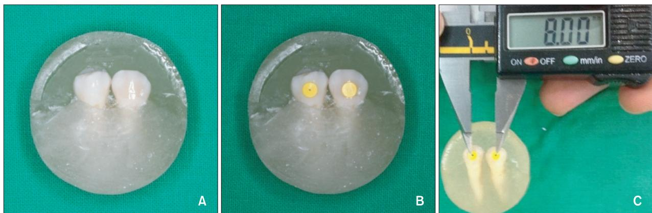
**Figure 1.** The experimental sample. A, One pair of teeth embedded in a resin block. B, A sticker attached to the buccal surfaces of the sample teeth. C, The distance between the midpoints of 2 stickers (8 mm).
