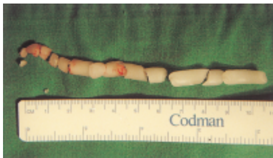
Fig. 3. The Miragel explant shows extreme friability and a tendency to disintegrate into fragments intra-operatively.
