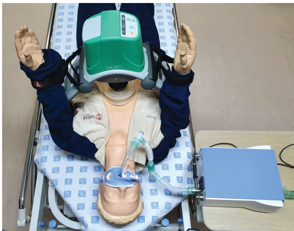
Fig. 1. Manikin model : CPR manikin with airway circuit connected to the flow analyzer. A mechanical chest compression device is installed in the manikin.
