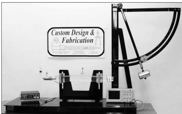
Fig. 3. Fluid percussion injury device developed by custom design and fabrication of virginia commonwealth university medical center.
