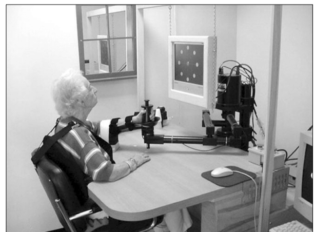
Fig. 1. Robot training with the MIT-Manus at the Burke Medical Research Institute. A patient seated in front of the Massachusetts Institute of Technology-Manus device with her shoulders strapped to the chair and moving the manipulandum. The patient's hand is strapped to a wrist carrier attached to the manipulandum. The video screen is above the training table.
