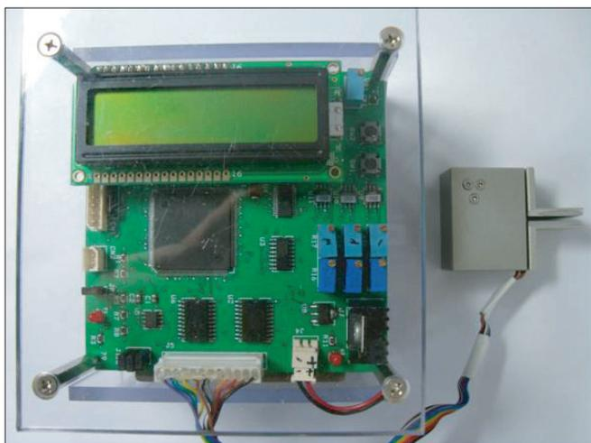
Fig. 1. Digitalized Pinch Dynamometer.
