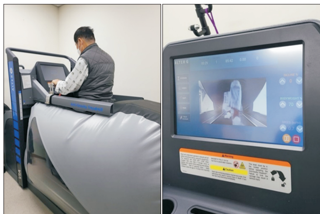
Fig. 1. Antigravity treadmill device. The device (Via model; AlterG Inc., Fremont, CA, USA) consists of a treadmill enclosed by a waist-high chamber, an air compressor that controls the internal pressure, and a monitoring screen.
