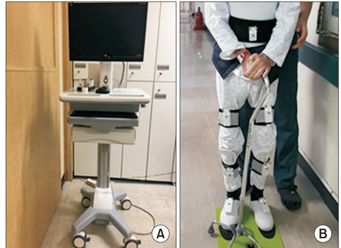
Fig. 1. (A) Gait analysis with inertial measurement unit technology, Human Track (RBioteck Co. Ltd., Seoul, Korea). (B) The IMU sensors are attached to patient's abdomen, bilateral thighs, shanks, and dorsum of both feet.
