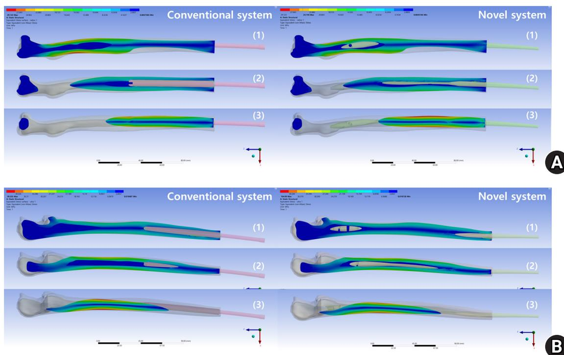
**Fig. 3.** Stress-distribution pattern when stress was loaded along the X-axis at the radius (A) and the ulna (B).
