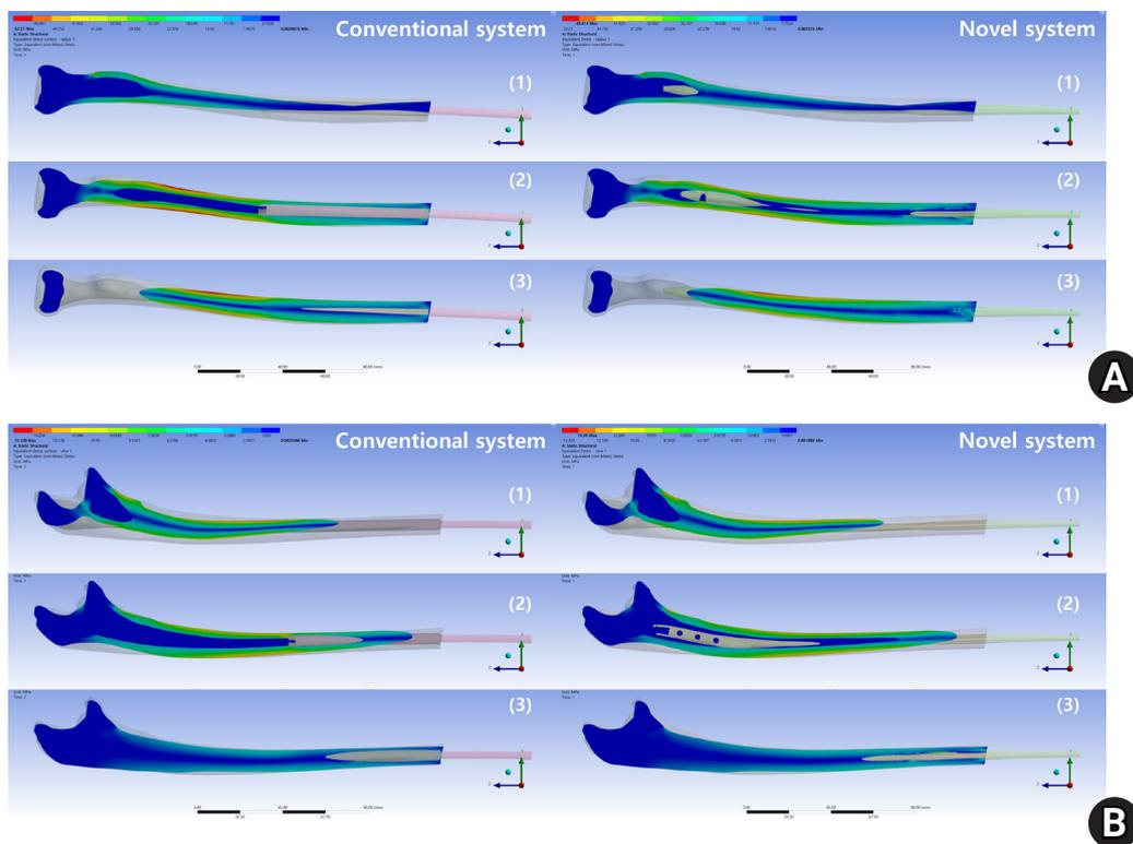
Fig. 4. Stress-distribution pattern when stress was loaded along the Y-axis at the radius (A) and the ulna (B).
