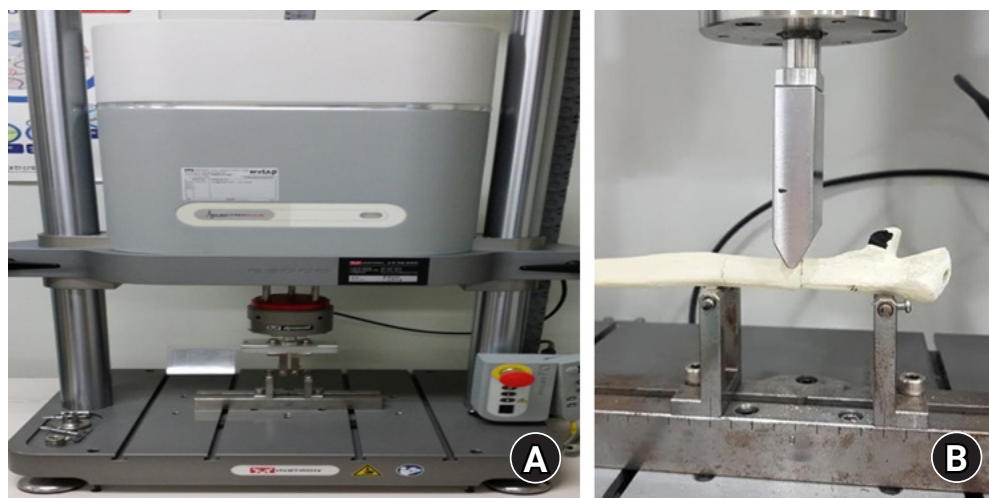
Fig. 2. (A) ElectroPuls E3000; Instron, Norwood, MA, USA. (B) Three-point bending test; span distance, 80 mm.
