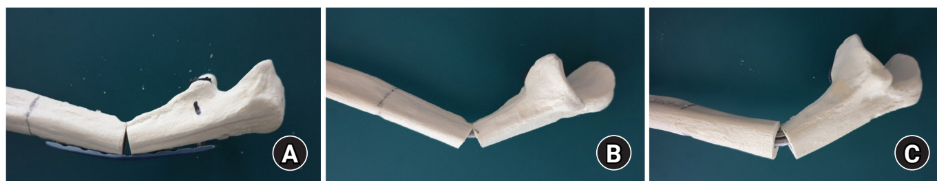
Fig. 3. Post experimental gross photos of sawbone fixed with each method. (A) Fixed with plate and screws. (B) Fixed with headless compression screw. (C) Fixed with Steinmann pins.
