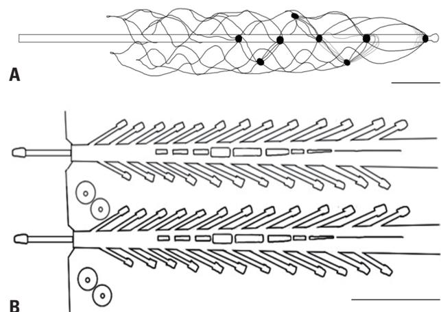
**Fig. 4.** Minimally invasive devices. (A) Stentrode with  $8 \times 750 \mu\text{m}$  electrode discs self-expanding during administration by a 4F catheter. Scale bar, 3 mm. The device is usually implanted in the superior sagittal sinus to obtain the electrical activity of the brain. Figure adapted from Oxley et al.<sup>17</sup> (B) Neural threads. "Tree" probes with electrode contacts spaced by  $75 \mu\text{m}$ . Scale bar,  $100 \mu\text{m}$ . Figure adapted from Musk.<sup>19</sup>
