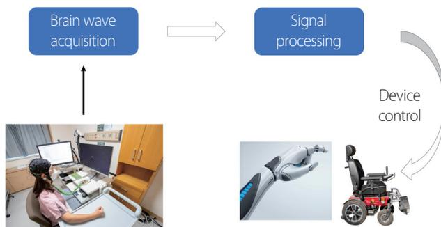
**Fig. 1.** Concept image of a brain-computer interface. Figure adapted from Wolpaw et al.<sup>21</sup>
