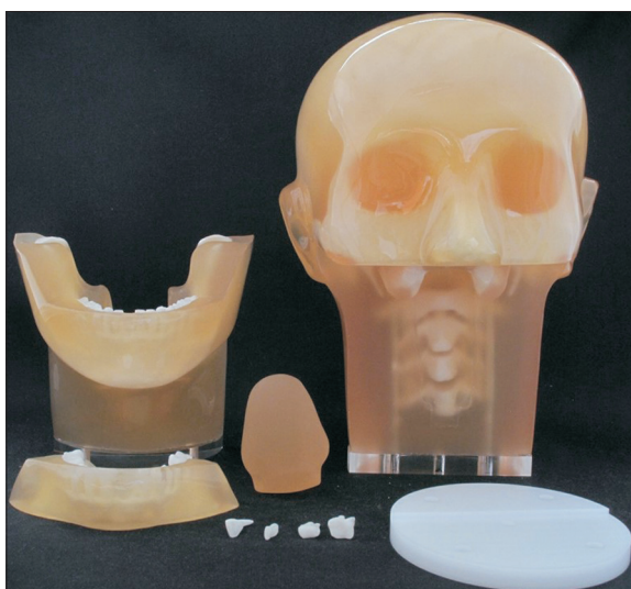
Fig. 1. Tooth extraction specifications for the dental head phantom. The maxillary/mandibular incisor, maxillary premolar, and maxillary molar models are removable, allowing fixation of the extracted teeth.
