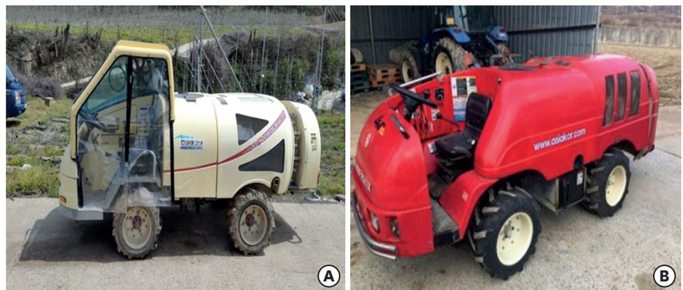
**Fig. 2.** (A) A cabin-style speed sprayer. (B) A cabinless-style speed sprayer.
