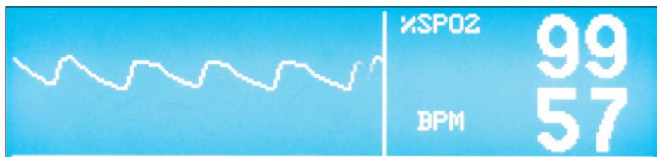
Fig. 1. Good waveform on pulse oximeter.
