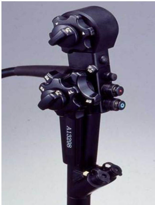
**Fig. 1.** GIF-2TQ260M (Olympus Medical Systems Corp., Tokyo, Japan). Second bending section overcomes some of the limitations of flexibility inherent with standard endoscopes when approaching anatomically difficult lesions for endoscopic submucosal dissection (ESD).
