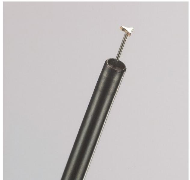
**Fig. 3.** Triangle-tipped (TT) knife (Olympus, Tokyo, Japan).
