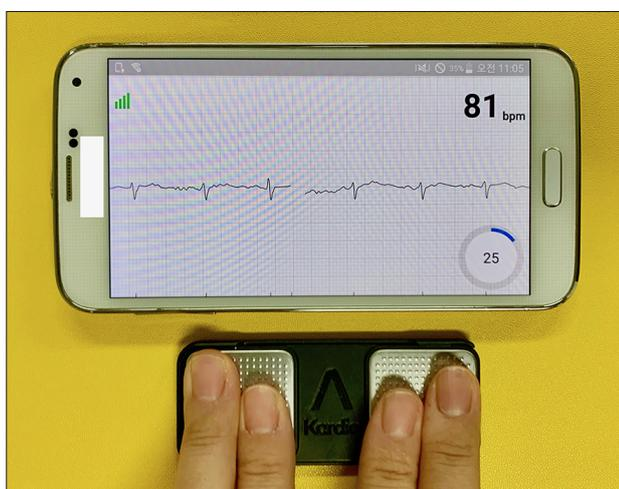
**FIG. 1.** Kardia Mobile Heart Monitor. The electrocardiogram appears on the display of the smartphone.
