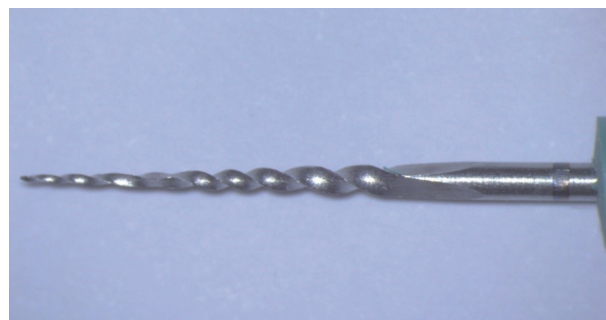
Fig. 2. TF instrument showing unwinding.
