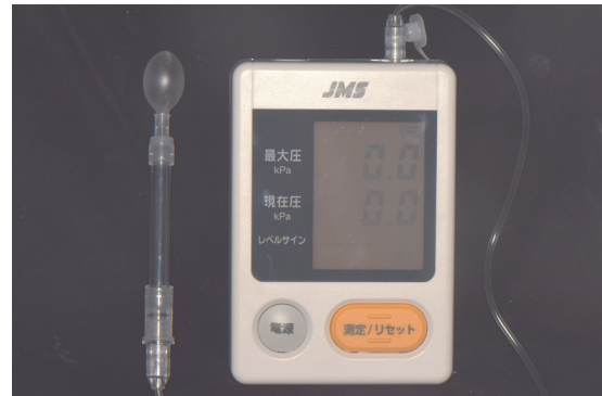
Fig. 6. A tongue pressure-measuring device (JMS tongue pressure measurement device™).
