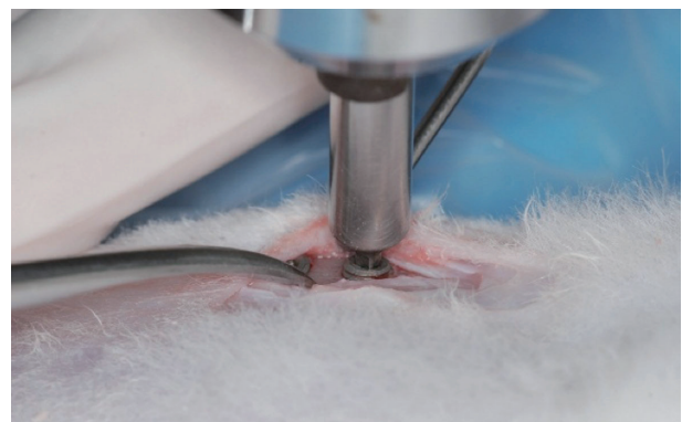
Fig. 3. Removal torque were measured by digital torque gauge.
