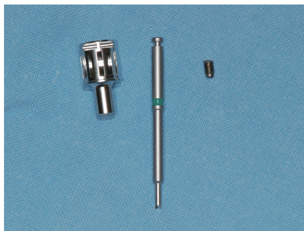
Fig. 4. Removed abutment screw & used fork-shaped end driver.
