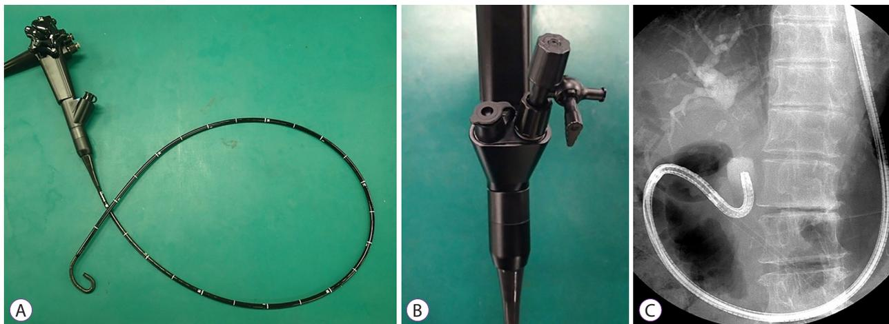
**Fig. 4.** Prototype of a multibending ultra-slim scope. (A) The distal end has two bending sections for facilitating biliary insertion. (B) Two accessory channels (2.2 and 1 mm) designed to facilitate irrigation during intraductal lithotripsy. (C) Free-hand bile duct insertion of the scope. (Picture courtesy of Prof. Jong H. Moon, MD, PhD, FASGE, FJGES, Director of Digestive Disease Center, SoonChunHyang University School of Medicine, Bucheon/Seoul, Korea).
