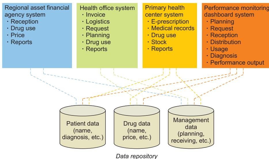
Figure 2. Description of the information systems before service-oriented architecture (SOA) was applied.
