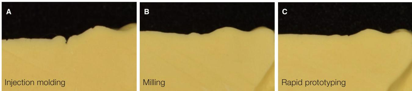
**Fig. 10.** Cross-sectional view of the palatine rugae reproduced with impression materials. (A) Injection molding method, (B) Milling method, (C) Rapid prototyping method.
