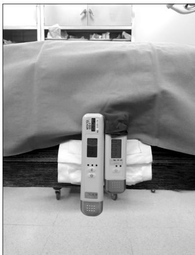
**Fig. 2.** The position of the two dosimeters at the side of the table. One dosimeter was wrapped with a radiation-reducing glove. Only one layer of the piece totally covered the radiation sensor of the dosimeter. Sensors were facing the patient and table.
