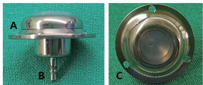
**Fig. 1.** Photographs of the V-Port. The V-Port is constituted of (A) a non-collapsible reservoir outlined with a titanium cage and (B) a connector for the ventricular catheter to be assembled. (C) The three holes of the titanium outer leaflet are designed to secure the V-Port on the skull using mini screws.
