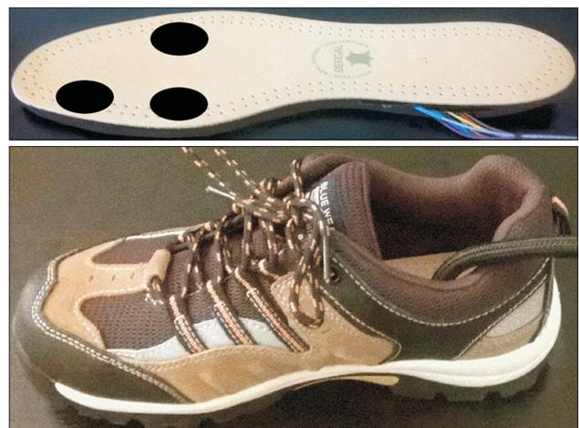
Figure 1. The locations of the three force sensors, under the cork and leather layer, are shown as black ellipses.
