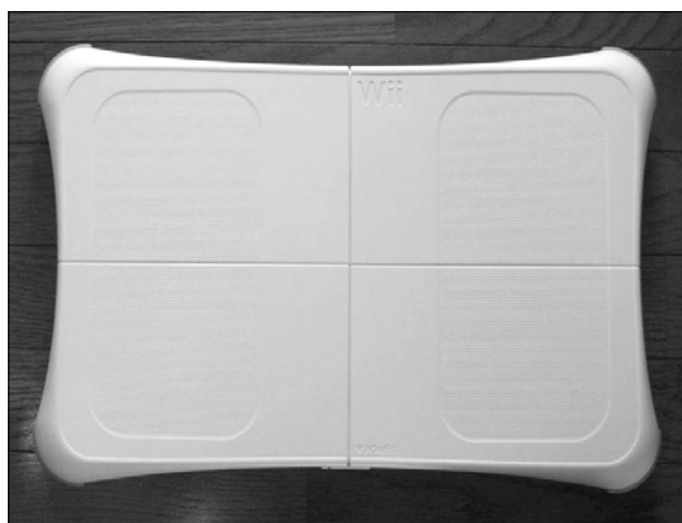
Fig. 3. The wii-fit balance board system has bluetooth and contains multiple pressure sensors that are used to measure the user's COP (center of pressure)-the location of the intersection between an imaginary line drawn vertically through the center of mass and the surface of the balance board and weight. The sensors on the board can accurately measure up to 150 kg (330 pounds).
