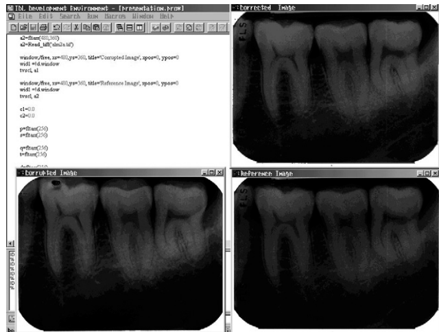
Fig 2. Image pairs(lower left and right) and contrast-corrected image(upper right), using the procedure written with IDL
